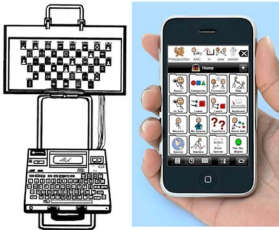
Figure 1. Left: the Words+ Portable Voice II system, as pictured in Romski and Sevcik (1996), utilized a cart so it could be wheeled around. Right: the Apple iPhone 3G with Proloquo2Go in the palm of a hand.
